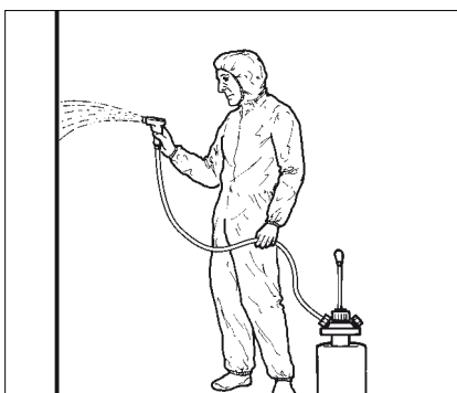
Use low-pressure spraying where possible
